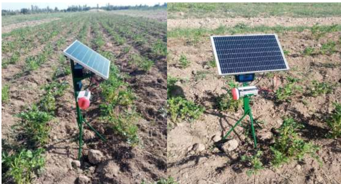
Figure 2. Installation of the solar-powered ultrasonic device in a potato field
