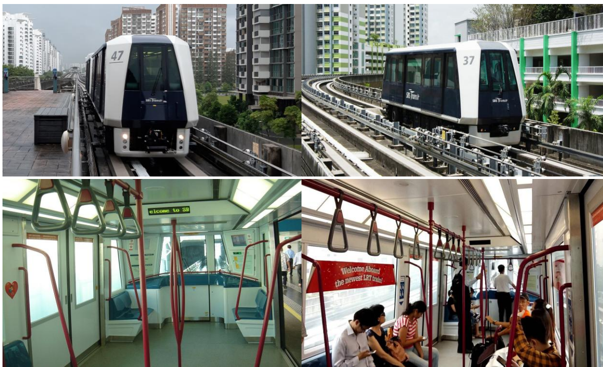
2-rasm. To‘liq GoA4 darajasidagi “Mitsubishi heavy industries crystal mover C810/C810A” elektr poyezdi.
