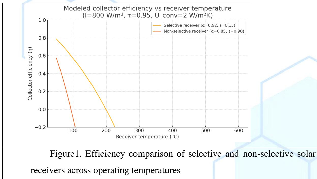
The graph (figure 1) illustrates how these two surface types behave across different receiver temperatures. The selective surface maintains higher efficiency across the full temperature range, while the non-selective surface loses performance rapidly. This pattern reflects the strong impact of thermal emission at elevated temperatures and highlights the importance of selective coatings for both medium- and high-temperature solar thermal devices.
