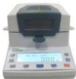
Figure 1. Determination of the concentration of the chemical admixture using a moisture analyzer
