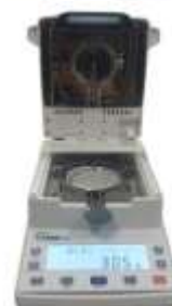
Figure 1. Determination of the concentration of the chemical admixture using a moisture analyzer
