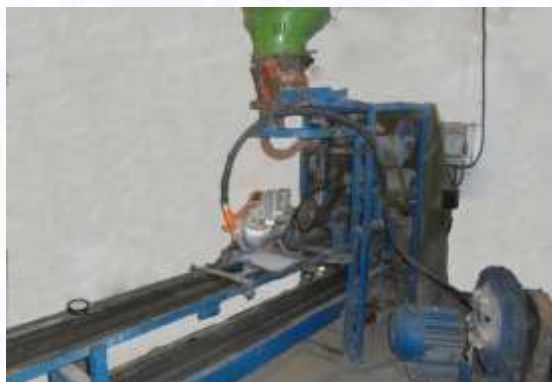
Fig. 1. Universal stand designed for testing machines for planting
